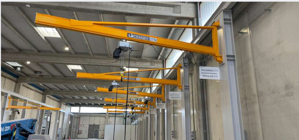
Project for 11 1Tn. wall-mounted jib cranes.
